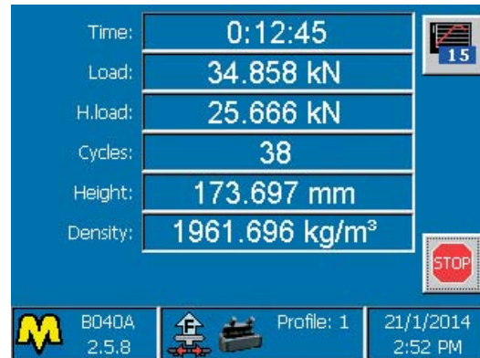
Test parameters during compaction
