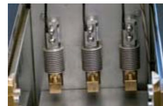
Detail: 3 load cells 500 N
