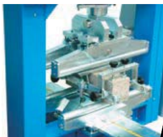
C090-15 + C109-15N fixed on the flexural machine C090-07N
