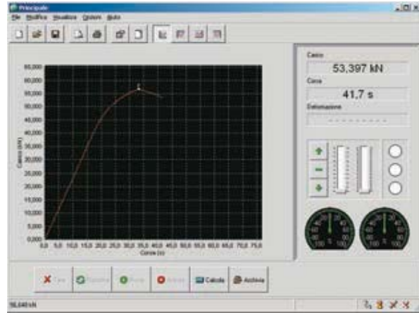
C109-12 Graphic of splitting tensile test execution
