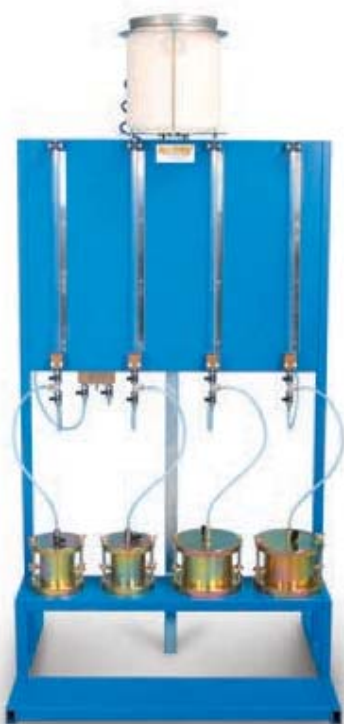
S248 with permeameters
